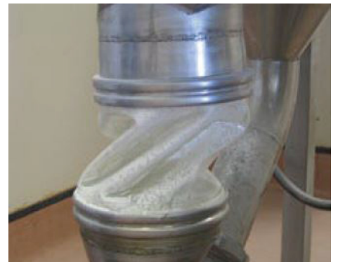
INSTALLATION GAP TOO WIDE
